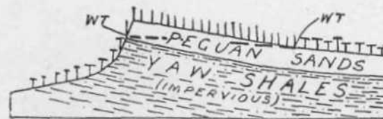
Fig(j. 10. Section showing details of the central part of Fig. 9. WT=water table. Rain falling on the ridge sinks rapidly through the porous sand (hence the dry Indaing. I) but lower down at the points marked WT and WT hence the moister Teak Forest. L. D. S.
